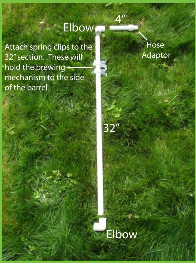
Using PVC primer, thoroughly clean the connection points of the PVC pipes and elbows. Then, using PVC cement, connect the various parts as illustrated above.
