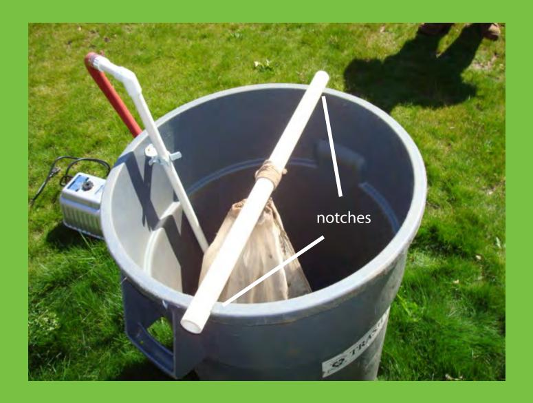
To secure the PVC pipe that will lay across the barrel and suspend the bag of compost, cut two notches in each side of the pipe as illustrated above. Attach bag of compost to the pipe then lay pipe across top of barrel.
