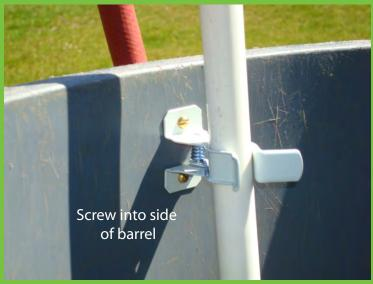
Place brewer inside trash barrel. Drill two ¼" holes in the side of the barrel so that the holes line up with the spring clips attached to the 32" PVC pipe. Using screws, attach the brewer to the side of the barrel so that the brewer is suspended approximately 6" off the bottom of the barrel.
