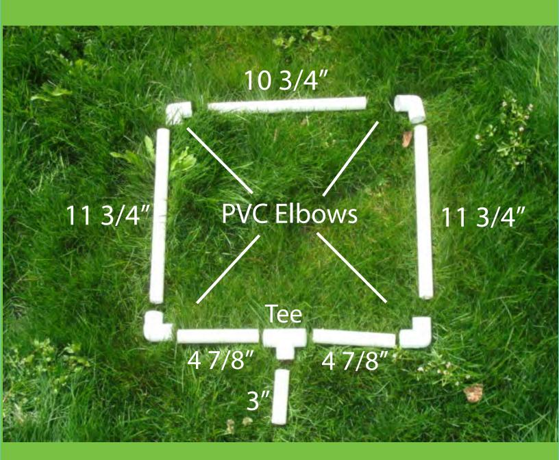
Using PVC primer, thoroughly clean the connection points on the pipes and elbows. Then, using PVC cement, connect the various parts as illustrated above.
