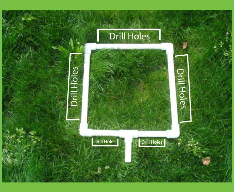
Drill 1/8" holes every inch or so along the tops of the areas of the pipes illustrated above.
